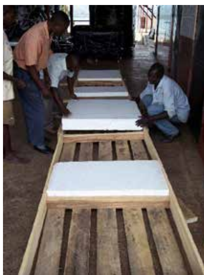
(c) Floating wooden platform
